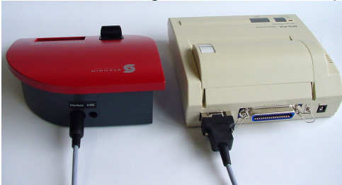
Illustration 33: Connecting the Seiko DPU-414 printer.
