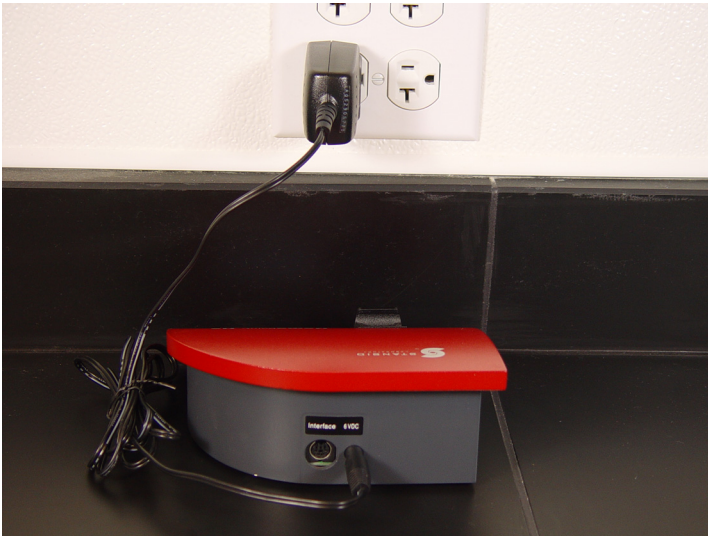
Illustration 3: Connecting the power adaptor.
