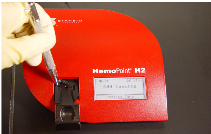
Illustration 34: Removing the cuvette holder.
